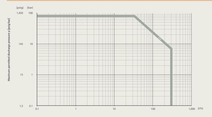
Flow rate  $Q_{\text{theor}}$  per pump head at maximum stroke [gph/l/h]
